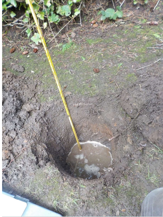
Photo 7 Piezometer ground water encountered in level test pit 2
