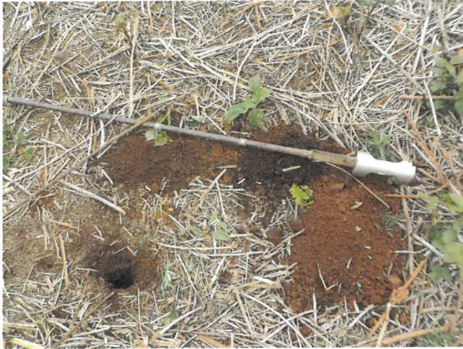
Photo 7 – View of the material encountered in hand augered boring B-3.
