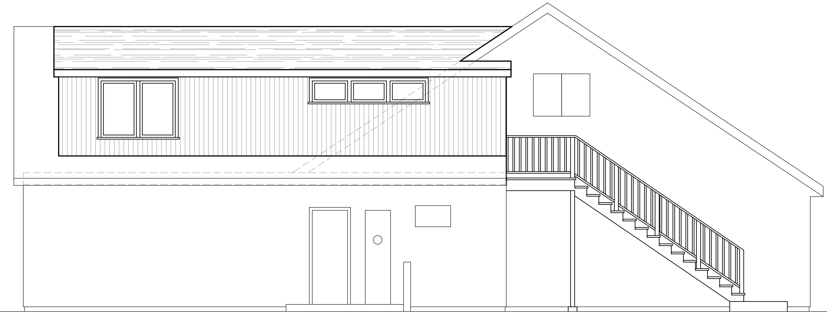
2 partial side (east) elevation A2.1 1/4"=1'-0" whalecove_xplan2.dwg
