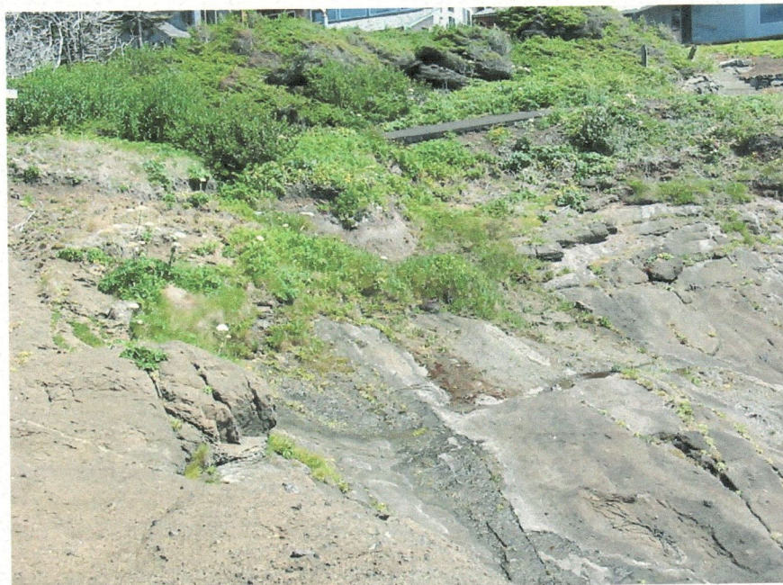
Photo 4 - Looking south toward basalt rock exposed along the upper part of the bluff slope. Springs emanate from some of the fractures in the rock.
